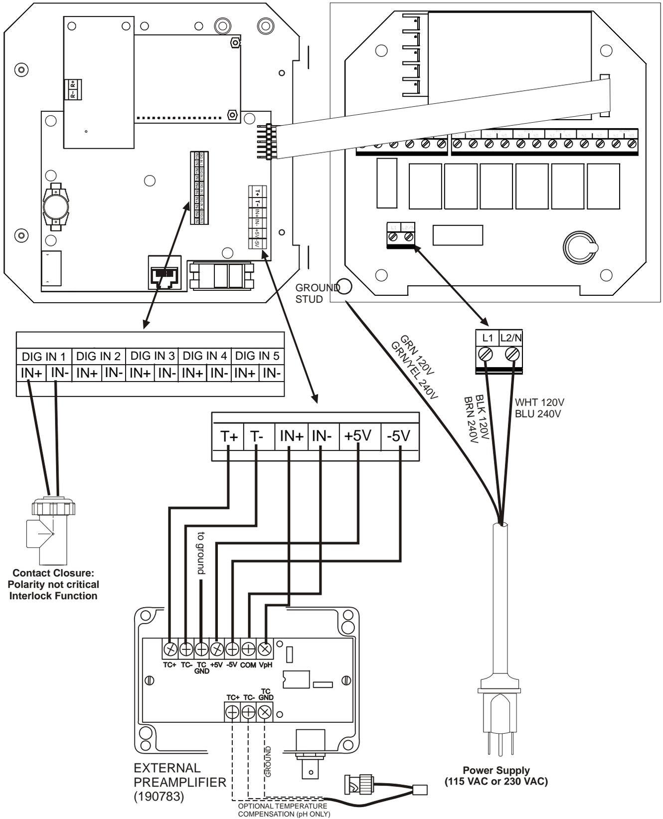
**Figure 3b WPH Inputs using pH/ORP Electrode/External Preamplifiers**
