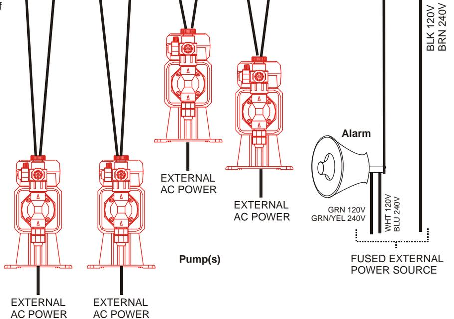
**Figure 4d WDP440 Outputs**
