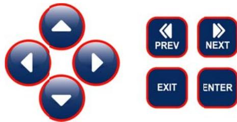
To change a value in a submenu, the left/right arrow keys move the cursor left and right to each digit or option that can be changed. The up/down arrows will change numeric values up or down, or scroll through option choices. Press **ENTER** only when you have finished making all of the changes for that menu screen.
