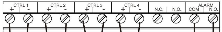
Note: The Alarm relay is not programmable. Refer to the Main Menu diagram for the list of error conditions that trigger the Alarm relay.
