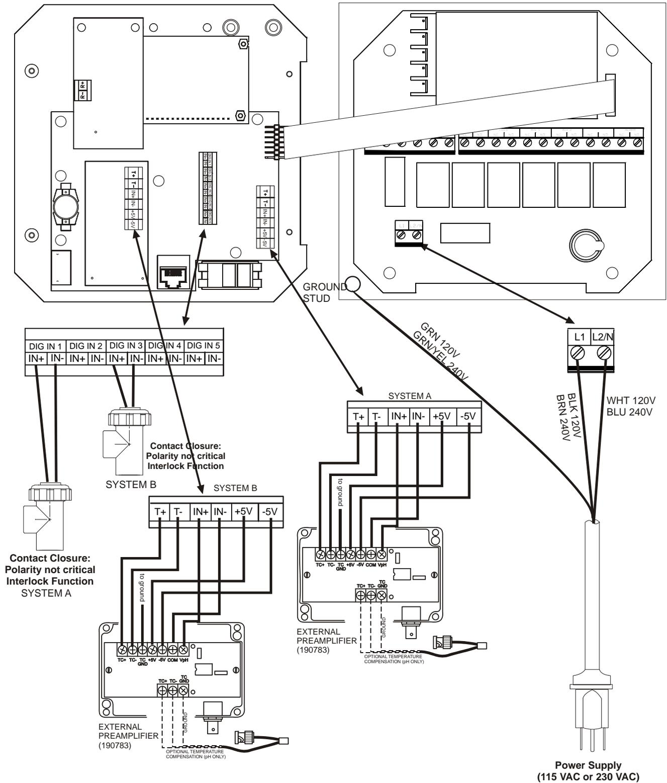
**Figure 3d WDP Inputs using pH/ORP Electrode/External Preamplifiers**
