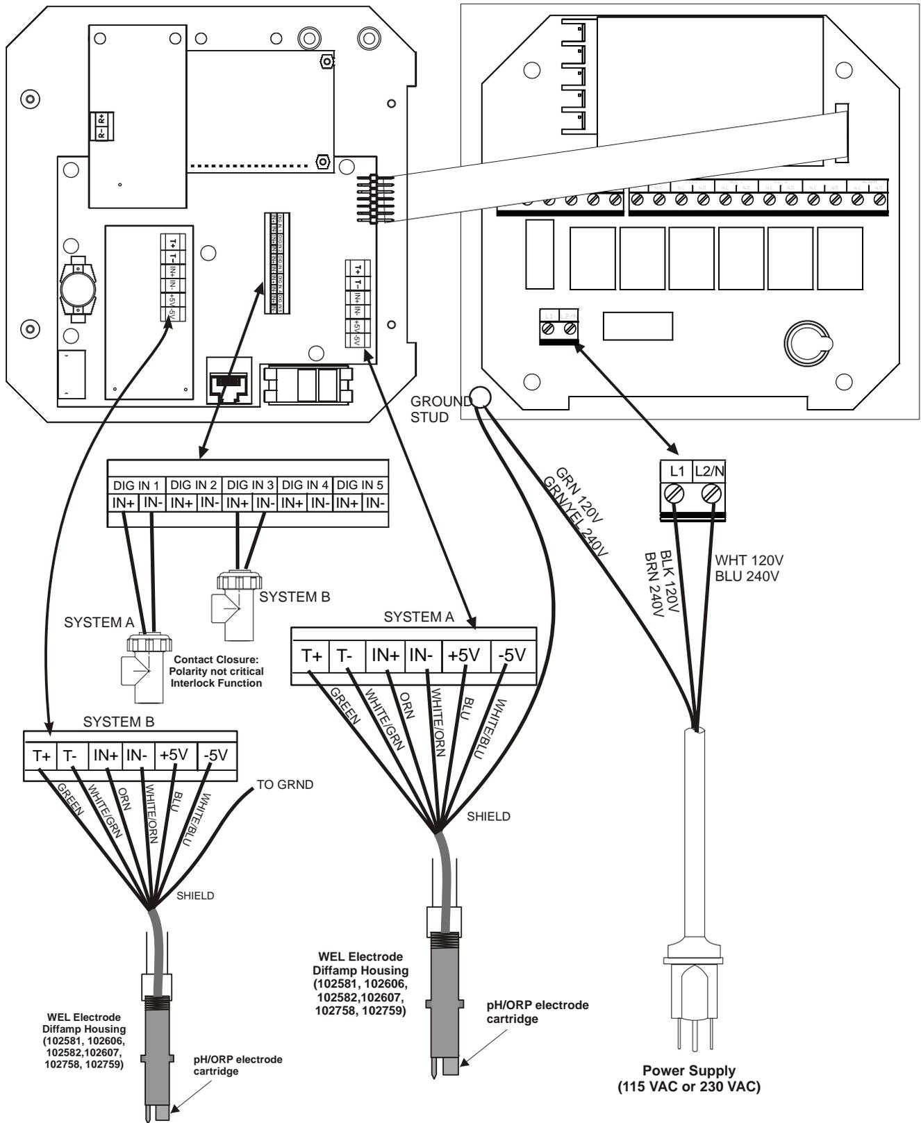
**Figure 3c WDP Inputs using WEL pH/ORP Electrode Housings**
