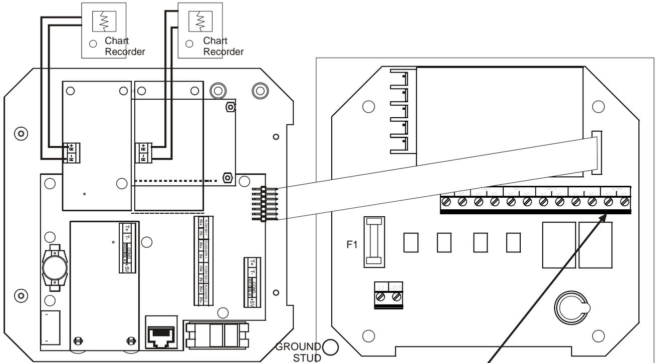
Note: Alarm is a dry contact relay (polarity not critical).
